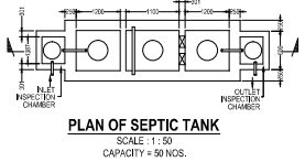
PLAN OF SEPTIC TANK CAPACITY = 50 NOS. SCALE = 1:50
